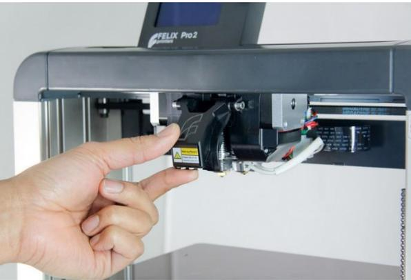
6. Remove hot-end connector of the corresponding hot-end.
